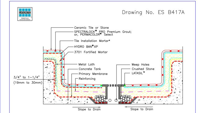
\*Tile Installation Mortar to be either 254 Platinum Plus, 254 Platinum , or MULTIMAX™ LITE.
