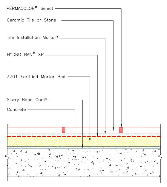
\* Slurry bond coat and tile installation mortar to be either 254 Platinum Plus, 254 Platinum or MULTIMAX™ LITE.
