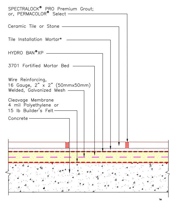
\* Tile installation mortar to be either 254 Platinum Plus, 254 Platinum or MULTIMAX™ LITE.
