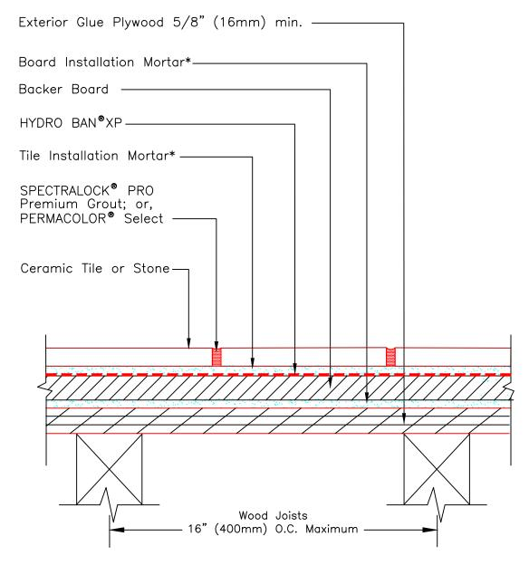
\* Board and tile installation mortar to be either 254 Platinum Plus, 254 Platinum ™or MULTIMAX LITE.
