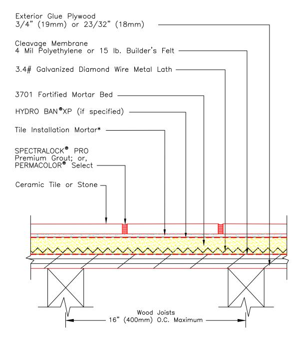
\* Tile installation mortar to be either 254 Platinum Plus, 254 Platinum or MULTIMAX™ LITE.
