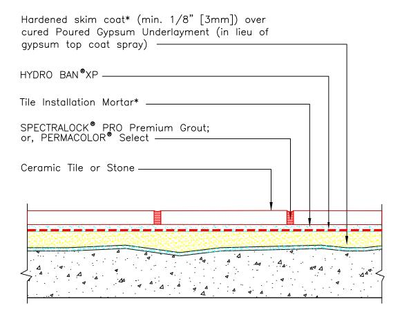
\* Skim coat and tile installation mortar to be either 254 Platinum Plus, 254 Platinum or MULTIMAX™ LITE. LATICRETE cannot warranty against cracking or water penetration if a LATICRETE waterproofing membrane is not installed.
