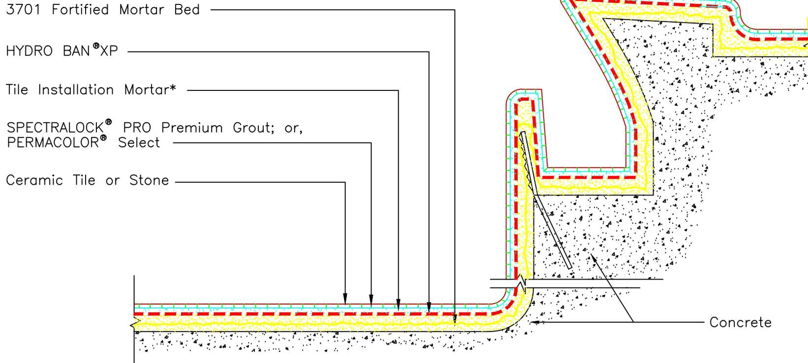
\* Slurry bond coat is required under the mortar bed at all horizontal surfaces. Slurry bond coat and tile installation mortar to be either 254 Platinum Plus, 254 Platinum or MULTIMAX™ LITE.
