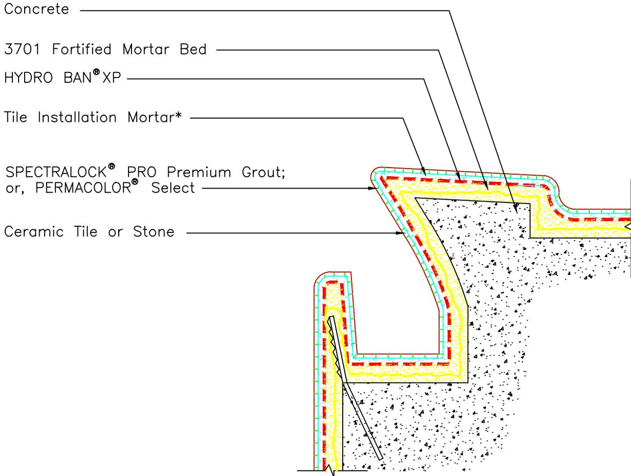
\* Slurry bond coat is required under the mortar bed at all horizontal surfaces. Slurry bond coat and tile installation mortar to be either 254 Platinum Plus, 254 Platinum or MULTIMAX™ LITE.
