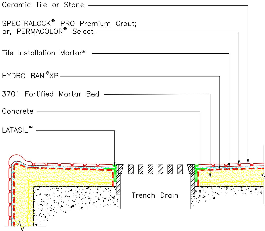
\* Slurry bond coat is required under the mortar bed at all horizontal surfaces. Slurry bond coat and tile installation mortar to be either 254 Platinum Plus, 254 Platinum or MULTIMAX™ LITE.
