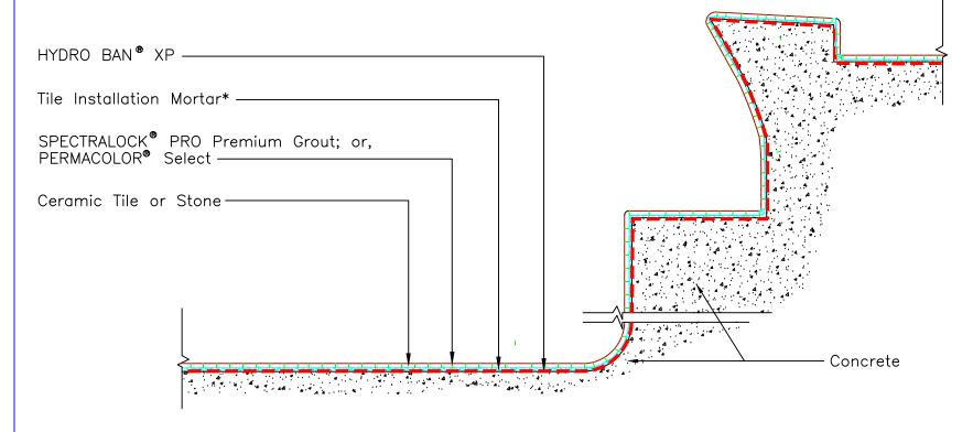
\* Slurry bond coat is required under the mortar bed at all horizontal surfaces. Slurry bond coat and tile installation mortar to be either 254 Platinum Plus, 2574 Platinum or MULTIMAX™ LITE.
