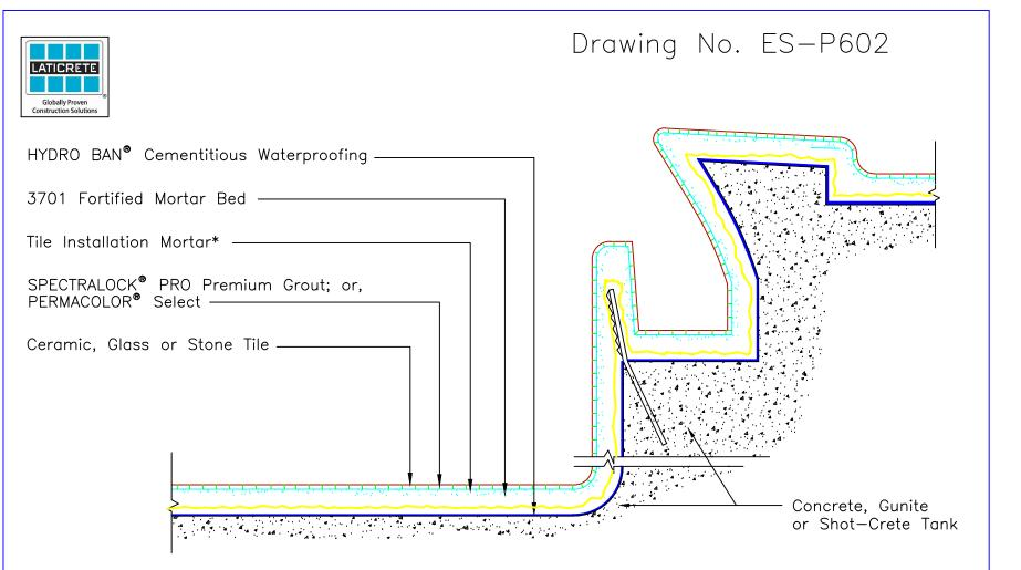
\* Slurry bond coat is required under the mortar bed at all horizontal surfaces. Slurry bond coat and tile installation mortar to be either 254 Platinum Plus, 254 Platinum or MULTIMAX LITE. Movement joints are required at all changes of plane, around all penetrations, and throughout field on floors and walls. Use LATICRETE LATASIL with LATICRETE 9118 Primer in movement joints. Refer to TCNA EJ-171 for more information on movement joints.
