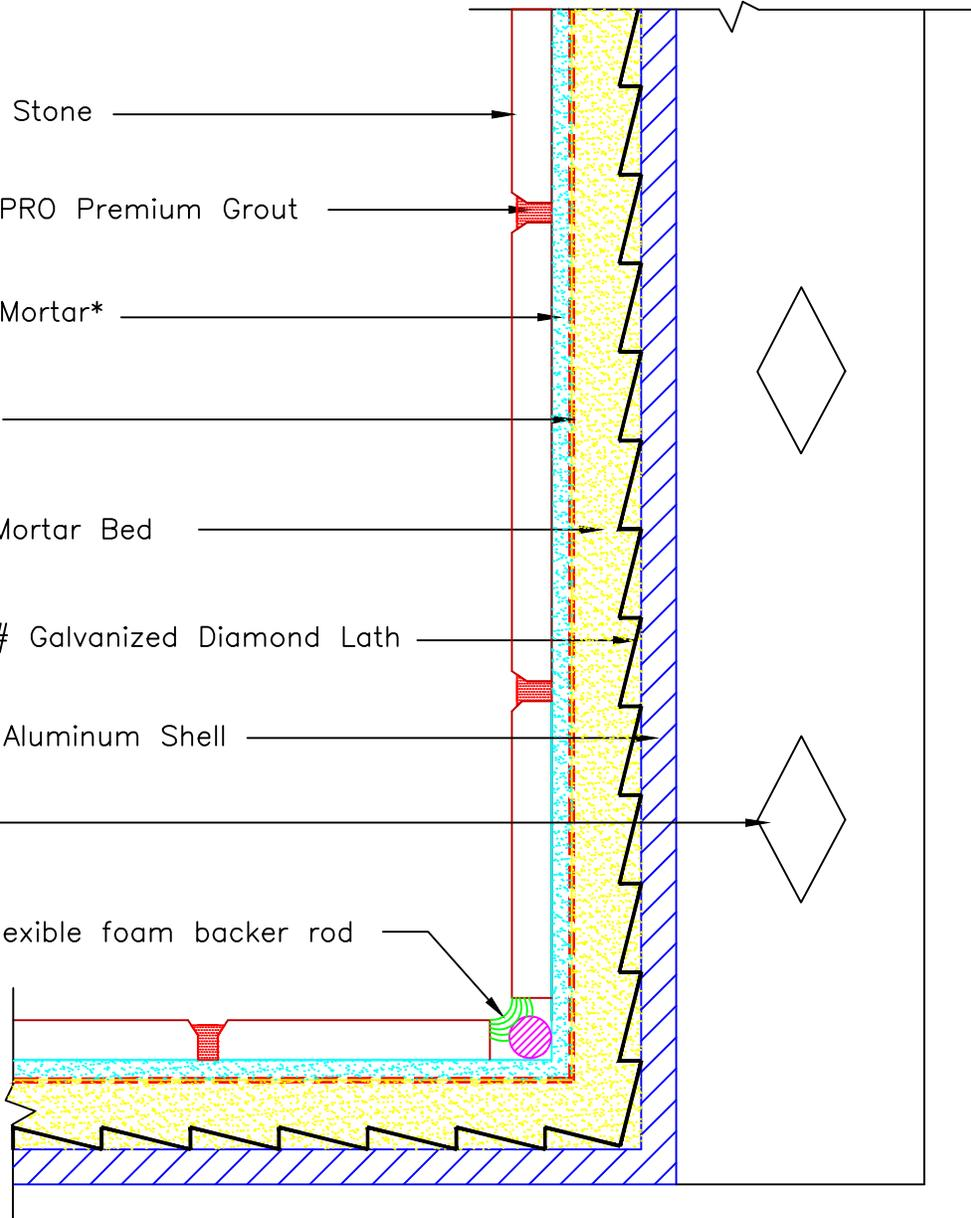
\* Tile installation mortar to be either 254 Platinum Plus, 254 Platinum or MULTIMAX™ LITE.
