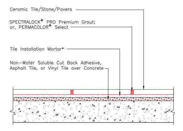
\* Tile installation mortar to be either 254 Platinum Plus, 254 Platinum or MULTIMAX™ ™ITE.
