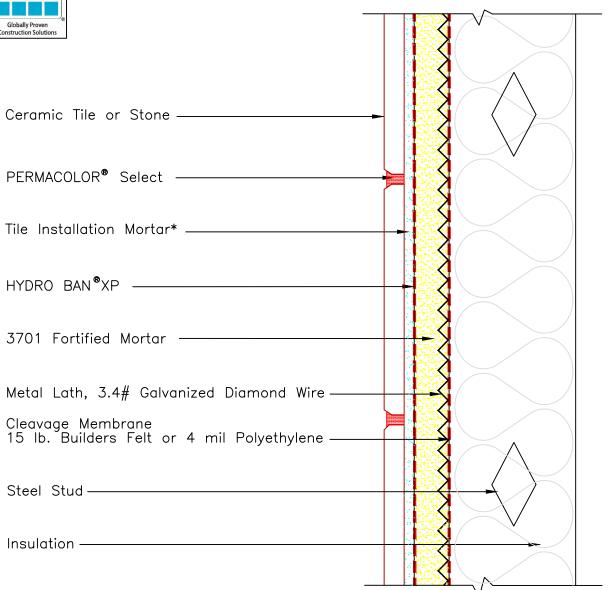
NOTE: Vapor Barrier, Weather Barrier, Separation Sheet, Insulation, Waterproofing, and Furring Type/Location to be Determined by Design Professional. Maximum Allowable Deflection Under All Live, Dead and Impact Loads, Including Concentrated Loads, Must Not Exceed L/600 Where L=Span Length. Design Professional to Ensure Compliance With Building Code(s). \* Tile installation mortar to be either 254 Platinum Plus, 254 Platinum or MULTIMAX™ LITE.
