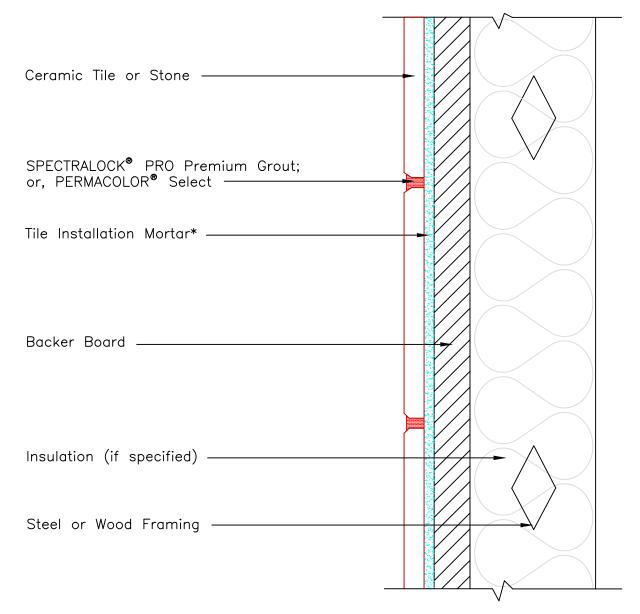
\* Tile installation mortar to be either 254 PLATINUM™ Plus, 254 Platinum or MULTIMAX™ LITE.
