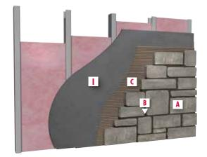
EXTERIOR WALL Concrete wall - lath with scratch and brown coat
