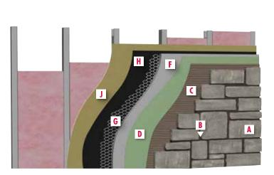
EXTERIOR WALL Framed wall with exterior rated sheating — lath with scratch and brown coat
