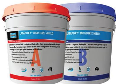
LATAPOXY® Moisture Shield is a two component, roller applied, breathable epoxy coating specifically designed to reduce moisture vapour emissions in concrete and other substrates. Use over dry and damp concrete and other masonry substrates to reduce the moisture vapour emission rate (MVER) in substrates to facilitate the installation of membranes, tiles, vinyl, timber, adhesives or other floor covering that require protection from moisture.
