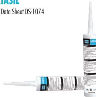
LATASIL™ sealant is a high performance, one component, neutral cure, 100% silicone sealant designed for ceramic tile and stone applications. Meets ASTM C290 Type S, Grade NS, Class 25, Use I, M & G. Equipped with fungicides to resist mould and mildew growth. Resistant to pool chemicals. Has excellent movement capacity - 25% extension and compression for movement joints. Use with LATASIL 9118 Primer in immersed installation and with porous stone.
