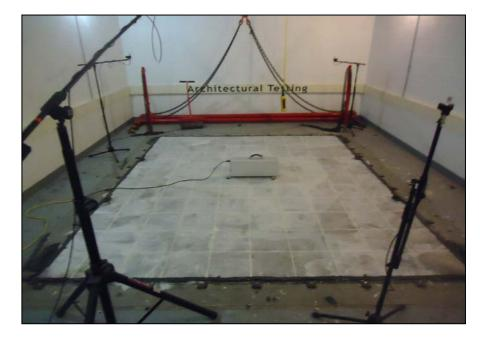
Source Room View of Test Specimen Installation
