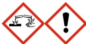
Corrosion Exclamation mark
