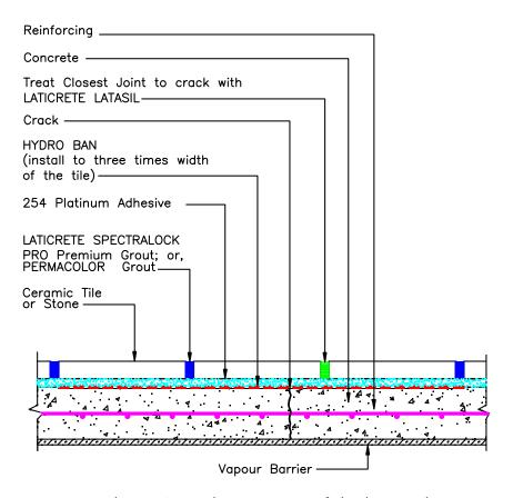
Detail AES F125a outlines treatment of shrinkage crack
