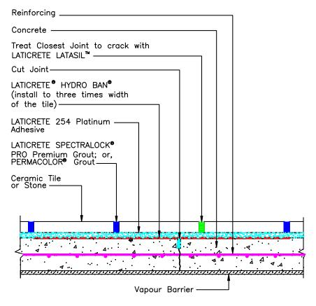
Detail AES F125b outlines treatment of saw cut or cold join in slab
