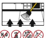
All surfaces should be between 60°F (16°C) and 90°F (32°C) and structurally sound, clean and free of all dirt, oil, grease, paint, concrete sealers or curing compounds. Rough or uneven concrete surfaces
