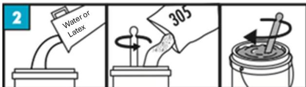
Place clean potable water into a clean pail, Add 305 Plus powder. Use approximately 4.2 - 4.6 liters of water or 3701 Mortar Admix (dilute 2 parts 3701 Mortar admix with 1 part water by volume), based on performance requirements. Mix by hand or with a slow speed mixer to a smooth, trowelable consistency. Allow mortar to slake for 5 – 10 minutes. Adjust consistency if necessary. Remix and apply with the proper sized notched trowel.
