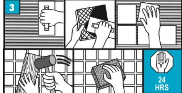
Apply mortar to the substrate with the flat side of the trowel, pressing firmly to work into surface. Comb on additional mortar with the notched side.
