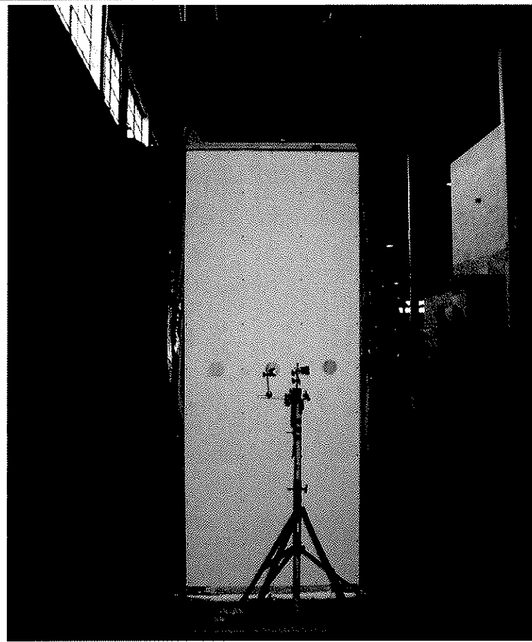
Structural performance test frame with wall assembly installed
