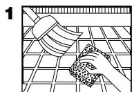
Before starting to grout remove spacers and debris in grout joints and remove dust and dirt using a damp sponge. Allow to dry. Do not leave water standing in joints. Do not clean tiles with acid cleaners. Substrate temperature must be between 45°F (7°C) and 90°F (32°C).
