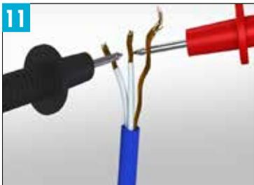
Test the resistance of the heating cable after tiling and check against previous values to ensure no damage has occurred.
