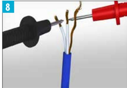
Measure the resistance of the STRATA\_HEAT Wire and verify it is still in line with the "Resistance Before" reading previously taken.
