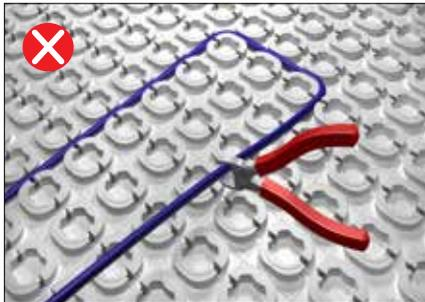
The STRATA\_HEAT Wire must not be cut, shortened, extended or left in a void, it must be fully installed within the layer of tile adhesive.
