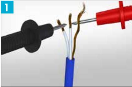
Measure and record the resistance of the STRATA\_HEAT™ Wire in the “Resistance Before” column of the control card, supplied as part of this installation guide on Page 32.
