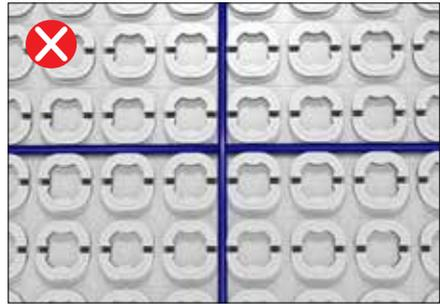
When installing the STRATA\_HEAT Wire DO NOT cross the wire over another run, over coldtails or the floor sensor. This will cause overheating and will damage the wire.
