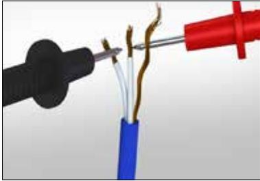
The STRATA\_HEAT™ Wire and floor sensors must be tested before they are laid, once they have been laid but before the tiles have been laid and again before they are connected to the thermostat. The resistance (ohms) of each heater should be measured. You should carry out the following tests and should expect the results detailed below:
