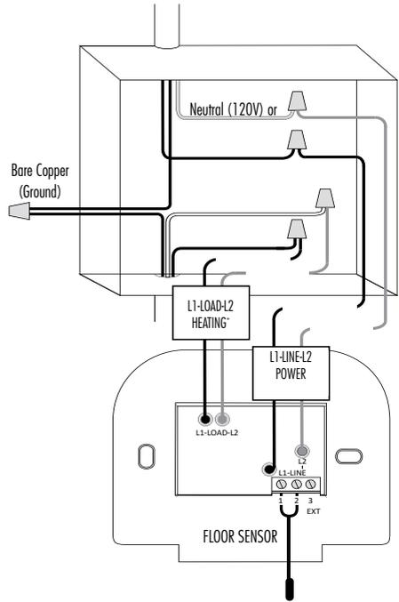
\*Undervoltage heaters are to be installed in parallel across the load terminals of the thermostat or contactor and must not exceed their rated load.
