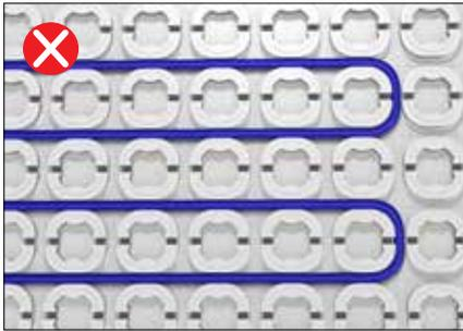
The standard spacing is 3 pegs (3 5/8") (92 mm) between parallel STRATA\_HEAT Wire. DO NOT install parallel runs of STRATA\_HEAT Wire closer than 3" (76.2 mm) if using cable spacing strips or 2 pegs (2 3/8") (61.2 mm) if using the STRATA\_HEAT Mat.
