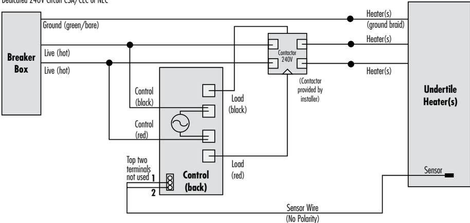
**NOTE:** All electrical work performed by a qualified electrician in accordance with local building and electrical codes and the Canadian Electrical Code, part 1 in Canada or the National Electrical Code in the USA, especially Article 424, Part V of the NEC ANSI/NFPA 70. Undertile heaters are to be installed in parallel across the load terminals of the thermostat or contactor and must not exceed their rated load.
