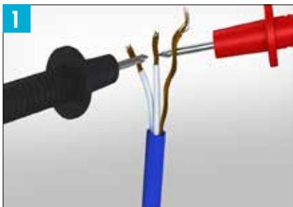
When the tiles have been installed, conduct another resistance test as described on Page 30 to ensure the sensor and STRATA\_HEAT Wire have not been damaged and record in the control card on Page 32.
