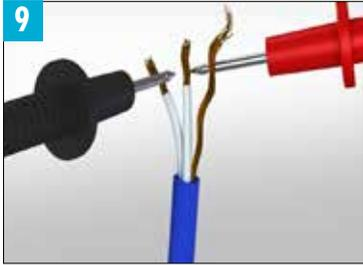
Test the resistance of the STRATA\_HEAT Wire after installation and check against the previous value to ensure no damage has occurred.
