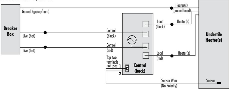
**NOTE:** All electrical work performed by a qualified electrician in accordance with local building and electrical codes and the Canadian Electrical Code, part 1 in Canada or the National Electrical Code in the USA, especially Article 424, Part V of the NEC ANSI/NFPA 70. Undertile heaters are to be installed in parallel across the load terminals of the thermostat or contactor and must not exceed their rated load.
