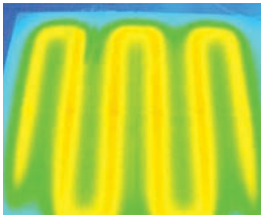
Infrared image using standard tile adhesive shows cold spots between wires
