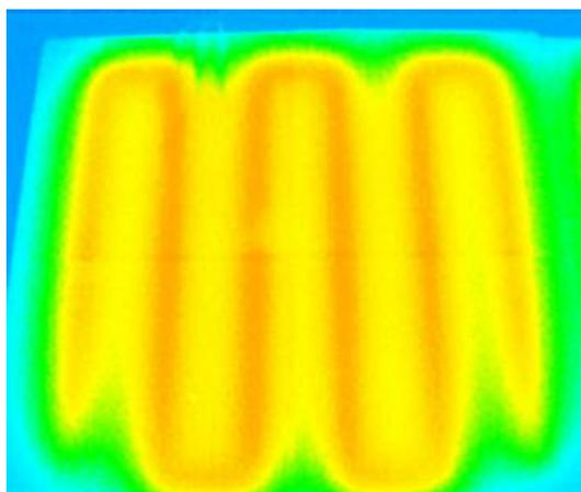
Infrared image using STRATA\_HEAT™ Thermal Pack<sup>1</sup> diffuses heat uniformly throughout — no cold spots
