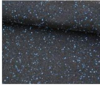
170.5 Sound & Crack Isolation Mat is a high performance acoustical underlayment system that muffles impact noises through ceramic tiles, stone and other hard surfacing materials. It also minimizes the transmission of cracks from the substrate to the tile installation up to 1/8" (3 mm) non-movement cracks. 170.5 Sound & Crack Isolation Mat is a 5 mm thick rubberized membrane comprised of 90% post-consumer recycled materials.
