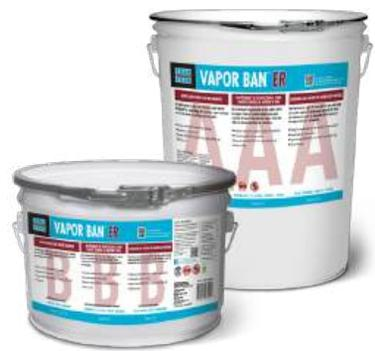
VAPOR BAN™ ER is a rapid curing, single-coat moisture vapor barrier designed for controlling the moisture vapor emission rate from new or existing concrete slabs. A two-part, 100% solids epoxy, it exceeds ASTM F3010 standard with a perm rating of 0.094 grains/h/ft<sup>2</sup> /in. Hg (5.4 ng/h • m<sup>2</sup> • Pa). VAPOR BAN ER is oil tolerant and can be applied by squeegee or roller.
