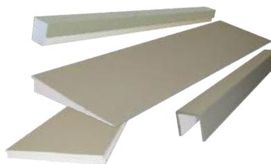
A wide range of accessories are available for the HYDRO BAN® Pre-Sloped Shower Pan. These accessories are all components of the expanded HYDRO BAN line of waterproof products that allow for high quality rapid shower installations. All of the HYDRO BAN Shower Pan Accessories are constructed of lightweight high-density expanded polystyrene with a waterproof finish and are ready to tile.
