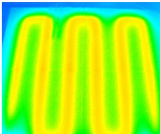
Infrared image using standard tile adhesive shows cold spots between wires
