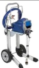
In addition to the conventional means of applying HYDRO BAN, the airless spraying technique can be used as an alternate means of application. HYDRO BAN can be effectively sprayed to increase productivity up to three times or four times on large projects. Any airless sprayer can be used that will deliver up to 3300 PSI (22.8 MPa) using a maximum tip size of 0.031" (0.79 mm). See TDS 410 for further information on the application of HYDRO BAN with an airless sprayer.
