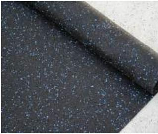
A 1/8" (3 mm) thick underlayment membrane that provides sound reduction and anti-fracture protection for tile or stone installations.
