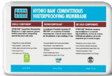
A one component, polymer fortified, cement based waterproofing material that mixes only with water. HYDRO BAN Cementitious Waterproofing Membrane handles negative and positive hydrostatic pressure up to 2 BARS (29 PSI) when applied at 40 Mils (1 mm) thick. Flood test within 2 hours. Passes ANSI A118.10 Waterproofing.
