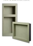
HYDRO BAN® Preformed Niche is a component of the expanded HYDRO BAN line of waterproof products that allow for high quality rapid shower installations. HYDRO BAN Preformed Niche is constructed of lightweight, highdensity expanded polystyrene with a waterproof finish and is ready to tile. Custom sizes available with a 4 week lead time from receipt of site drawing and Purchase Order. Contact your local LATICRETE Sales Rep for further information.
