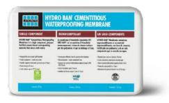
A one component, polymer fortified, cement based waterproofing material that mixes only with water. HYDRO BAN Cementitious Waterproofing Membrane handles negative and positive hydrostatic pressure up to 2 BARS (29 PSI) when applied at 40 Mils (1 mm) thick. Flood test within 2 hours. Passes ANSI A118.10 Waterproofing.
