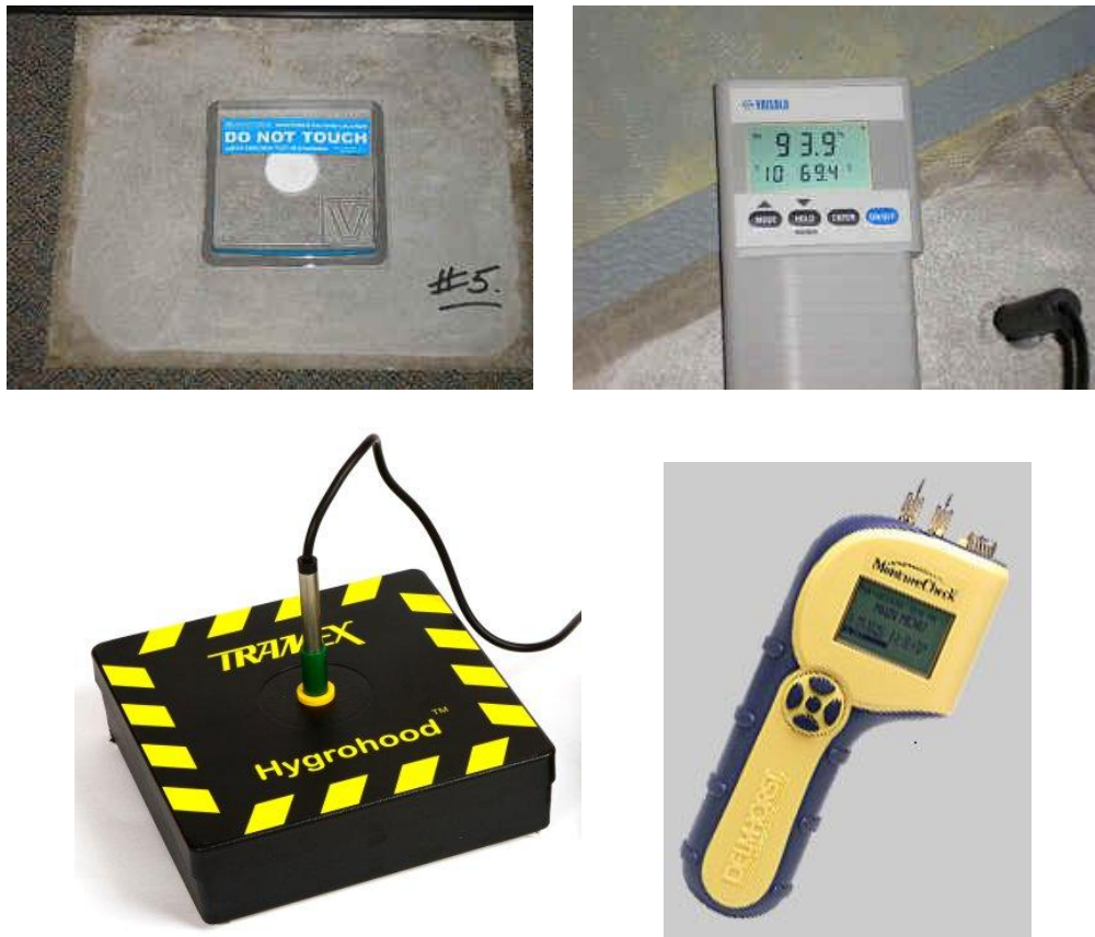
Figure 1.1 – (Clockwise from top left) ASTM F1869 Calcium Chloride Test Kit, ASTM F2170 Relative Humidity Meter, ASTM F2420 Insulated Hood with probe attached, and ASTM F2170 Pin Type Moisture Meter (Photos courtesy of George Donnelly Testing & Inspections at www.moisturetesting.com , www.tramexltd.com and Delmhorst Instrument Co. at www.delmhorst.com .)
