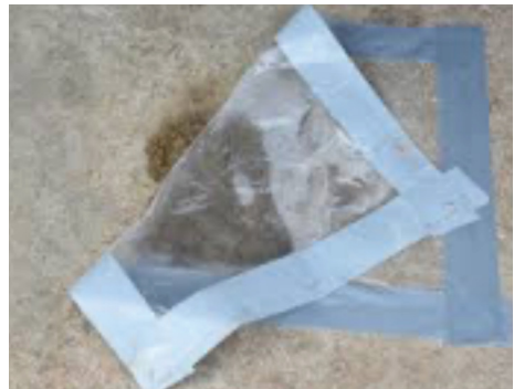
Figure 2.20 – ASTM D4263 – Plastic sheet method – 18" x 18" (45 cm x 45 cm) sheet of plastic is tightly taped to the substrate and allowed to sit undisturbed for 24 hours. If water or condensation is observed, then a measure of moisture vapor transmissions is present. This test will not provide a quantitative moisture vapor emission rate.
