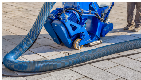
Figure 2.7 – Shot blasting machinery creates a concrete surface profile to improve adhesion and remove contaminants.
