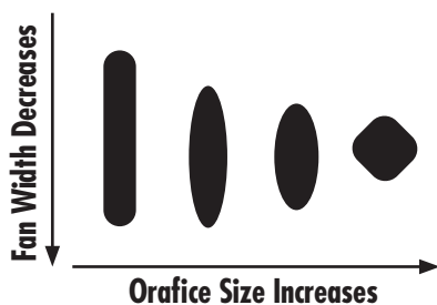
Figure 8.11 – Typical Spray Patterns of Liquid Applied Membranes.
