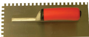
Figure 8.16 — A notched trowel has several important functions that contribute to a successful installation of ceramic tile and stone.
