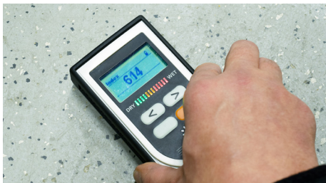
Figure 2.19 – In-Situ moisture testing.
