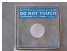
Figure 2.5 – ASTM F1869 calcium chloride test kit and ASTM F2170 Relative Humidity Meter.
