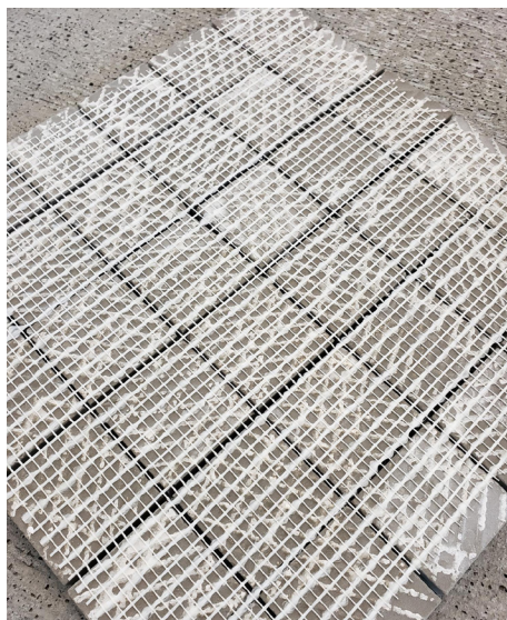
Figure 8.5 – Example of resin backed stone. Polyester resin mesh backing applied to the stone. Notice how easily the backing has peeled away from the stone itself.
