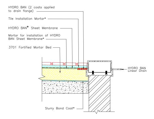
NOTE: This detail is intended to show installation of LATICRETE products and is not to be used to show steam room construction, placement of insulation, type of finish, structural considerations, or other design features. \*Slurry bond coat, tile installation mortar and mortar for installation of HYDRO BAN Sheet Membrane to be either 257 TITANIUM™, 254 Platinum or MULTIMAX™ LITE.
