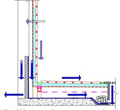
Figure 3.5.1 — Movement of moisture in a steam room application without insulation, low perm waterproofing membrane or vapor diffusion retarder.
