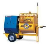
Figure 5.7.2 — Rotating Blade Type Mixer.
