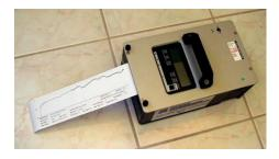
Figure 4.2.1 The BOT-3000 DCOF AcuTest Method apparatus<sup>32</sup>
