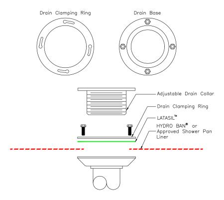
NOTE: It is important to ensure that drain weep holes are not blocked and are functioning fully.
