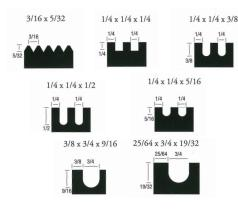
Figure 5.8.2 Notched trowel sizes for installation of adhesive mortars.
