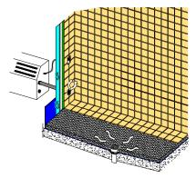
Figure 3.5.5 — How steam enters steam room and the condensate water evacuates.
