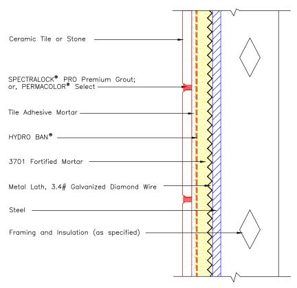
Note: Slurry bond coat, tile installation mortar and mortar for installation of HYDRO BAN Sheet Membrane to be either 257 TITANIUM $^{\rm IM}$ , 254 Platinum or MULTIMAX $^{\rm IM}$  LITE.
