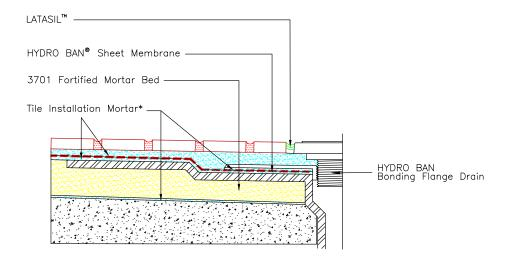
NOTE: This detail is intended to show installation of LATICRETE products and is not to be used to show steam room construction, placement of insulation, type of finish, structural considerations, or other design features. \*Slurry bond coat, tile installation mortar and mortar for installation of HYDRO BAN Sheet Membrane to be either 257 TITANIUM™, 254 Platinum or MULTIMAX™ LITE
