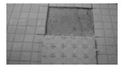
Figure 12.11 – Large PVC dots on rear/edge mounted porcelain mosaic tiles can lead to bonding issues as is evidenced from these photos. Latex fortified portland cement based thin set mortars may have a difficult time achieving a sufficient bond to the PVC rubber. The PVC dots are covering 50 – 60% of the tile back. An epoxy adhesive may be required to install tile mounted in this fashion in wet area and continuous submersion applications.
